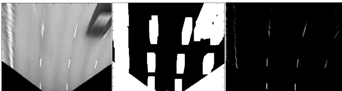
Figure 16. Left. Original image after IPM. Middle. Pavement detection. Right. Line detection.
